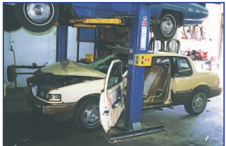
The aftermath of a student's failure to follow instructions. After the forward motion of the vehicle pinned a student between a work table and the wall and impaled his leg with a metal piece of the table, 3 more students were injured when the vehicle was reversed and wedged against the hoist.
